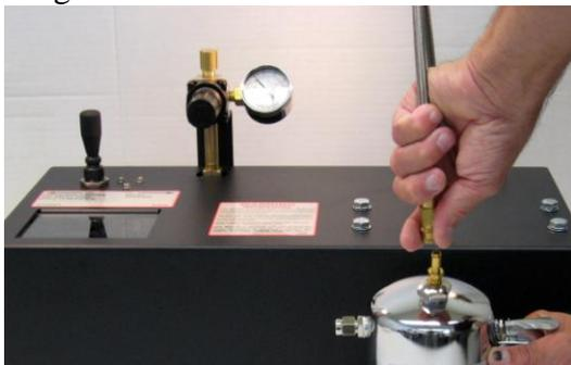
2. **Push the control lever to the right for liquid**, until the yellow cap on the rod (visible through the Plexi glass) reaches the red end mark on the label. Approx. 15 Seconds (Diagram 6). Let the lever return to center for several seconds. Then push the control lever to the left and hold for 15 seconds. This will siphon the first filling of chemical into the cylinder.
