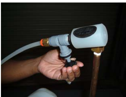
Opening the needle valve
