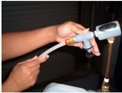
Connecting the air hose
